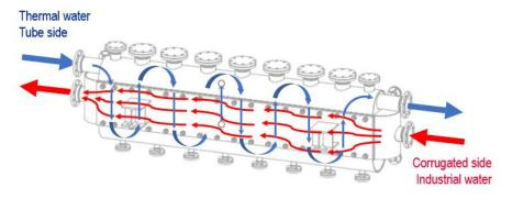
Moreover, the thermal water contains many salts, which makes it highly prone to plaque formation. For this reason, it is fed through the easy-to-clean tube side of the plate packs. Since the tubes are vertical, they are easily
