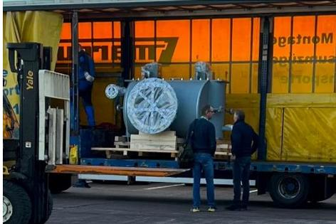
A global specialty chemicals company based in North Rhine-Westphalia needed a replacement condenser for an oxo plant. Since our hybrid could be integrated very well into the existing infrastructure and the low pressure losses required by the customer could be realized with it, we received the order. The recently delivered vacuum condenser weighs about 3.5 tons and offers an output of 867 kW on a heating surface of 163 m<sup>2</sup>. Vapors and water are fed in counterflow.
