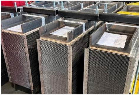
Similarly, the retrofit of an evaporator in a sugar factory in Baden-Württemberg is to be carried out at the beginning of next year. For this purpose, the existing Robert evaporator will be replaced by a much more efficient Hybrid Tubular falling film plate evaporator. The fully welded plate packs will have a heating surface of 4,400 m<sup>2</sup> and are already in production.
