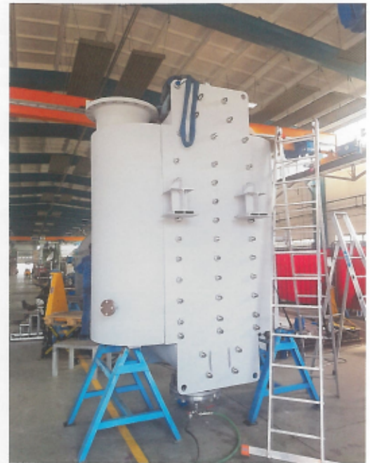
Figure 4. Pressure test preparation of a Hybrid tubular heat condenser in the production hall
